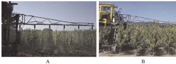
Fig. 1. Spray deposition and coverage test on (A) 2-year-old and (B) 3-year-old 'Autumn Spire' red maple liner plots with the high ground clearance sprayer (Tracker; GK Machine, Donald, OR).
